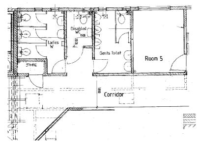
The drawing on the left shows how will change things proposed Phase 2 work. The main features are the wider corridor and the toilets split into three sections. The corridor is increased to about twice its current width (the dashed lines near the word 'Corridor' show the present width). You should be able to make out the bottom of the new stairs at the left-hand end of the corridor. The wider corridor much will be more inviting, encouraging people to move more
