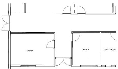
entrance doors have been moved about 3 feet along towards Gloucester Road, taking out the window and the cupboard. The cupboard houses various care-taking items such as cleaning products and spare bulbs; these would have to be found another home. The contents of the table could be placed in racks on the wall.
